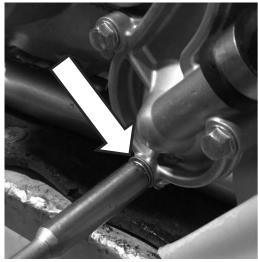
4. Remove the engine guard using a 10mm socket.
