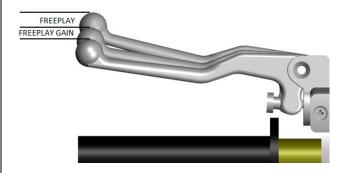
Optimal Free Play Gain yields 1/2-3/4" (12-19mm) of clutch lever movement, measured at the end of the lever. This measurement at the lever correlates to achieving the ideal installed-gap.
