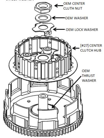
**NOTE**: If the OEM thrust washer is not in place, it is probably stuck to the backside of your OEM center clutch hub.
