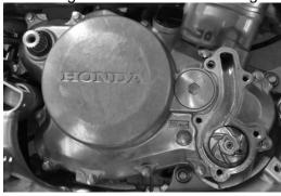
**NOTE**: Be sure that the copper washer for the water pump as well as the sleeve and O-ring for the water jacket are not displaced.
