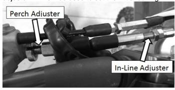
23. In the next section you will make adjustments using the front jam nut and perch adjuster to set the desired Installed-Gap based on the lever free play gain. Once this is established and everything functions well, you will tighten the adjuster jam nuts to secure your cable adjustment setting.
