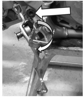
**8.** To avoid draining the oil, you can lay the motorcycle on its left side. Otherwise, stand the bike vertically on a center stand and drain the oil. In order to not spill oil the bike needs to be all the way down on its side. Catch any fuel that drains.
