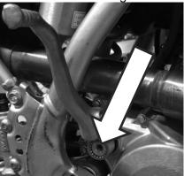
7. Remove the brake pedal bolt using an 8mm Hex Key and rotate the brake pedal away from the clutch cover.
