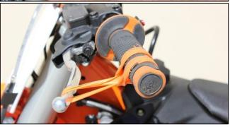
With the bike at idle in neutral, quickly blip (rev) the engine to at least half-throttle (~4,500 RPM) and let it return to idle. The end of the clutch lever should move in about 1/2-3/4" (12-19mm) toward the handlebar as you rev the engine.
