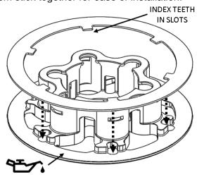
**17.** Install the pressure plate and lining plate assembly.
