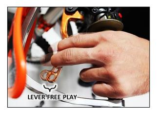
"Free Play Gain" is the increase of lever free play as the auto-clutch engages. This happens when the RPM increase from idle through around half-throttle (4,500 RPM). Free Play Gain is caused by the expansion of the EXP disk which lifts the pressure plate away from the throwout assembly.
